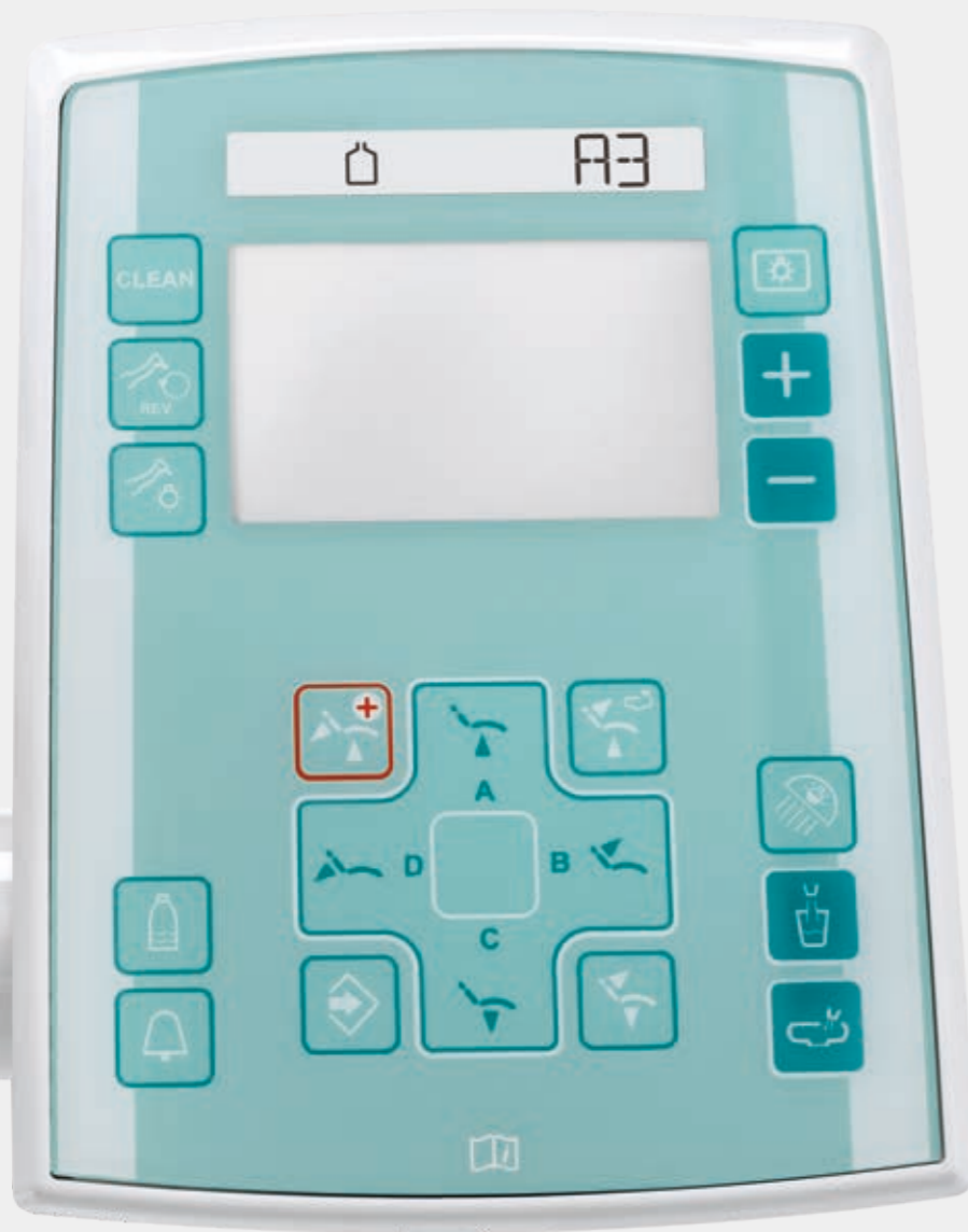
Touch screen display. The control panel surface, protected by capacitive glass, can be easily disinfected.
